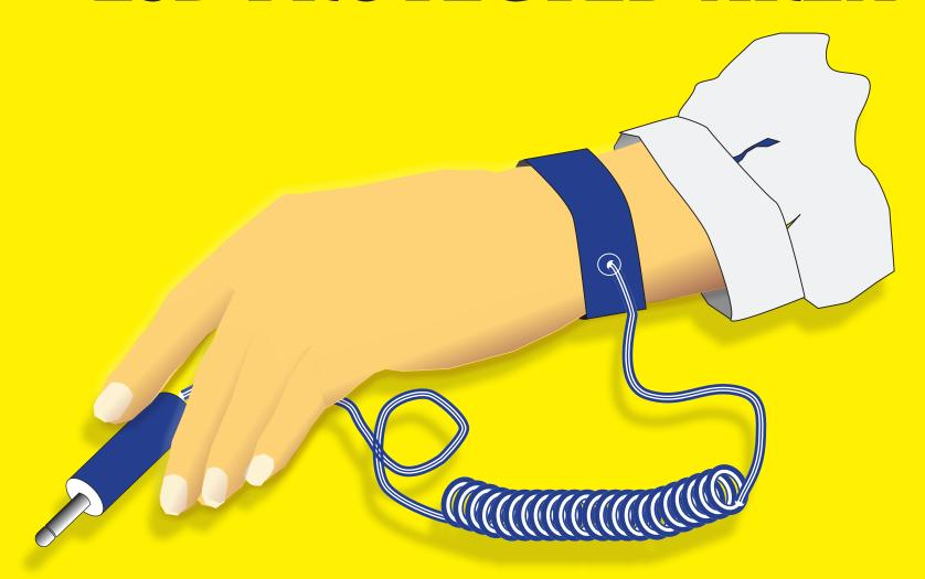
Verify that wrist strap is properly plugged in at workstation before handling any ESD sensitive devices.
