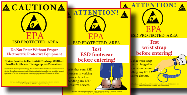
Three posters for display outside an EPA area to remind employees and visitors to test their equipment before entering.
