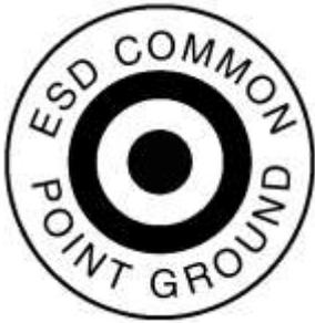
This ESD common point ground should be properly identified. ESD Association standard ANSI/ESD S8.1 – Symbols, recommends the use of the symbol in Figure 1 to identify the common point ground.
