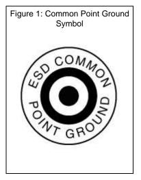
This ESD common point ground should be properly identified. ESD Association standard ANSI/ESD S8.1 – Symbols, recommends the use of the symbol in Figure 1 to identify the common point ground.
