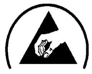
The ESD Susceptibility Symbol (Figure 3) consists of a triangle, a reaching hand, and a slash through the reaching hand. The triangle means "caution" and the slash through the reaching hand means "Don't touch." Because of its broad usage, the hand in the triangle has become associated with ESD and the symbol literally translates to "ESD sensitive stuff, don't touch."
