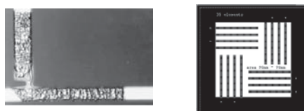
Figure 1. Typical photomask damage and layout of the CANARYESD™ test device
